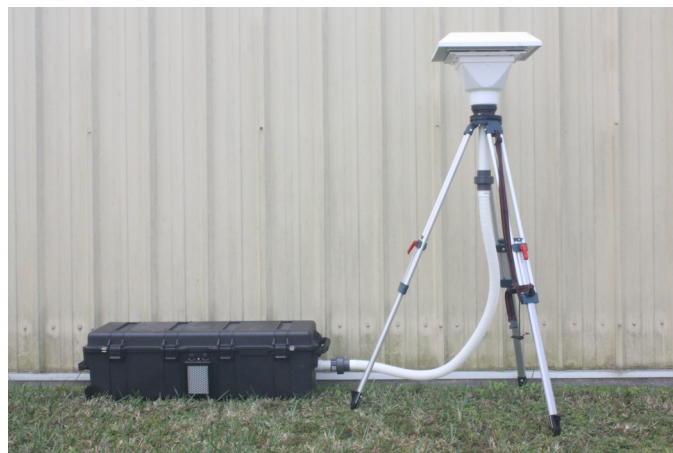
DF-ERHV-DT Digital Flow Meter Electronic Flow Management System Mobile High Volume Air Sampler
