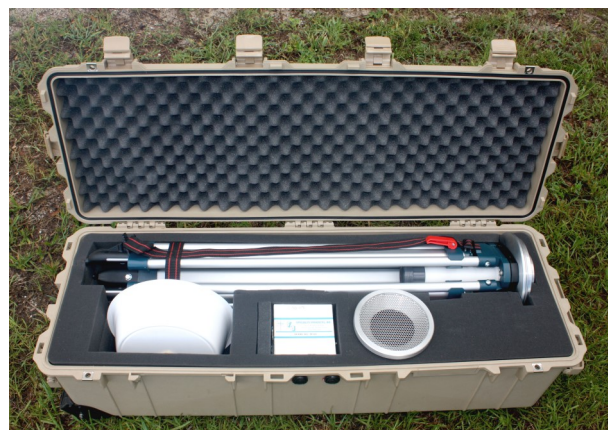
Transportation Storage Case for Tripod, Filter Holder with Rainshield, Particulate Filter Paper
