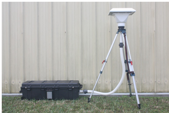
DF-ERHV-DTE Digital Flow Meter Electronic Flow Management System Mobile High Volume Air Sampler
