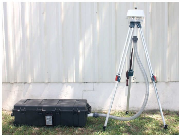
DF-ERHV-DTE-CFH Digital Flow Meter Electronic Flow Management System Mobile High Volume Air Sampler For Circular Filter Media
