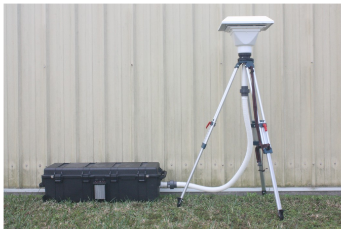
GAS-ERHV-DTE Global Air Sampler Electronic Flow Management System Mobile High Volume Air Sampler
