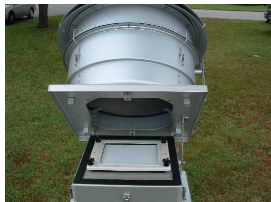
GAS-PM10DT Series System PM10 Inlet Open Position for Access to Filter Paper
