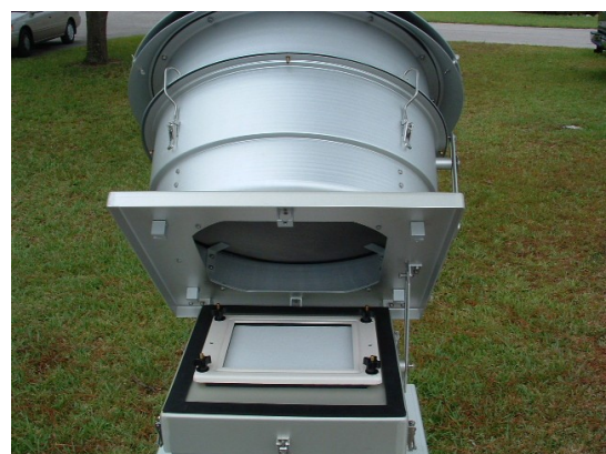
GAS-PM2.5DT Series System PM2.5 Inlet Open Position for Access to Filter Paper
