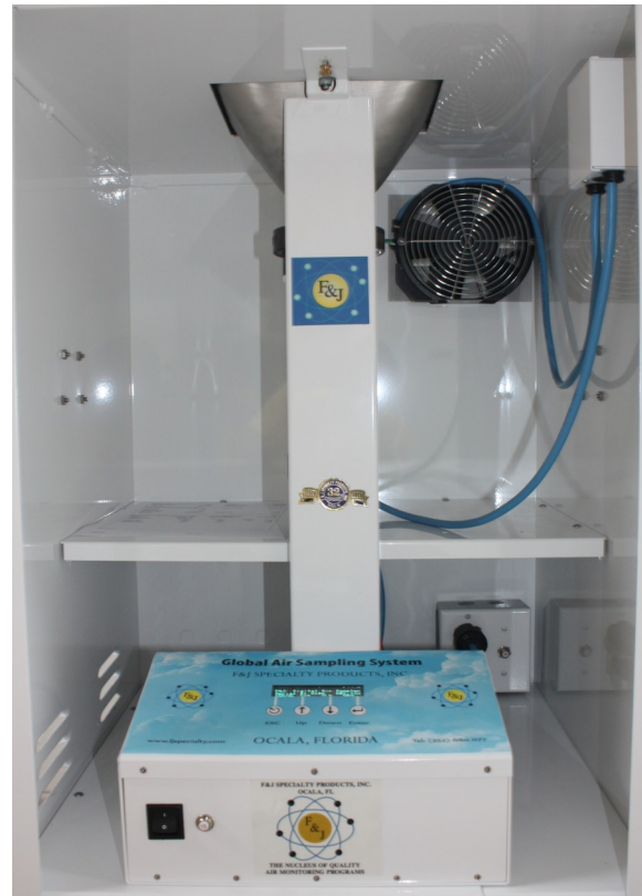
Close up frontal view of GAS-PM2.5DTE Series System enclosure interior
