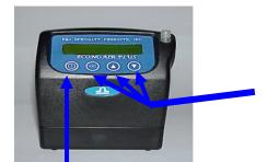
Press SET button and hold while using the Arrow keys to adjust flow
