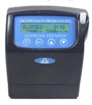
The F&J ECONOAIR Premium L-5PTR personal air sampler consists of a pump contained in a high impact steel fiber filled Lexan, antistatic and RFI/EMI-shielded case, exclusive electronic circuit board for constant flow control (patent pending), an LCD display with 2 lines of 16 characters, a single diaphragm pump mechanism and a rechargeable NiMH battery pack. The L-5PTR can be programmed for timing routine activated sampling.
